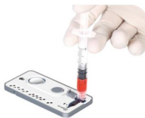
Step2: Fill the inlet with sample and slide the cap to seal the sample inlet.
